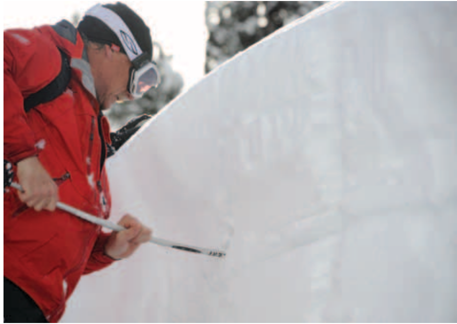
Mushroom test with a ski pole followed by a mushroom hand test. Below is a ski cut test on a small slope. Results and observations are then recorded.
